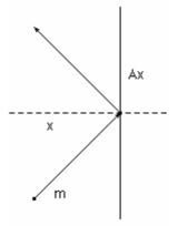
Elastic collision against a wall: the molecule "m" is reflected by the wall and forms equal angles of incidence and reflection.
